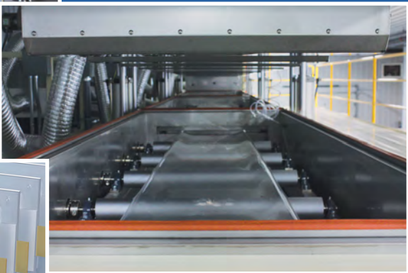
State-of-the-art clamshell roll support dryer
