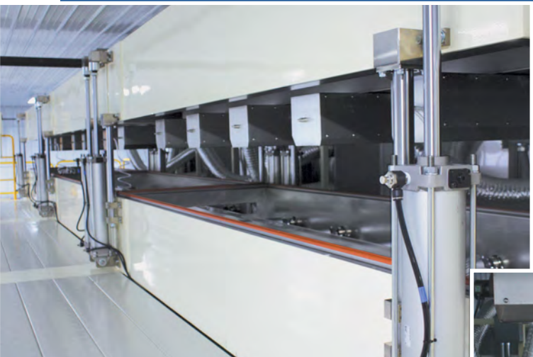
State-of-the-art clamshell roll support dryer
